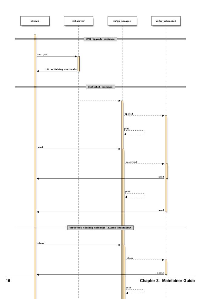
The initial connection is made by a WebSocket aware client to a WebSocket aware web server. The first exchange is dedicated to perform the upgrade handshake as defined by **RFC 6455#section-4**.
